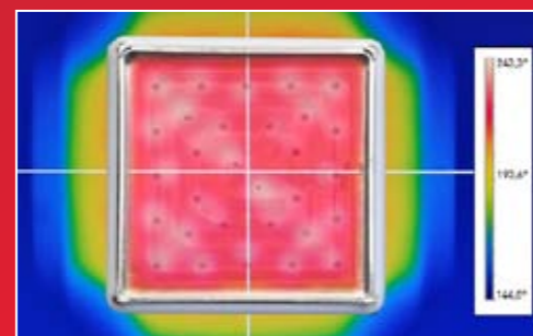
Optimal Temperature distribution of a BGA soldering tool
