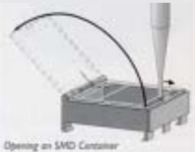
Opening an SMD Container
